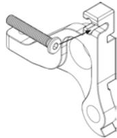
**Step 3:** Slide the Driveside Slider and Tension Screw into position on the driveside dropout. Thread the Tension Screw until the slider socket threads are positioned above the socket slot.
